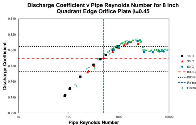
Figure 11: Discharge coefficient versus Reynolds number for 8 inch  $\beta=0.45$  QE orifice plate
