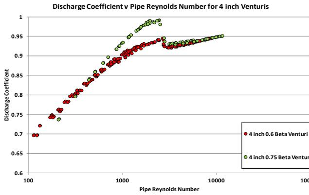
Figure 7: Discharge coefficient versus Reynolds number for 4 inch Venturis
