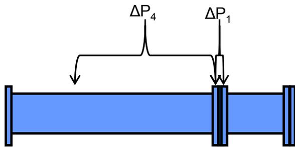
Figure 4: Orifice plate installed in a typical metering run (flow from left to right)
