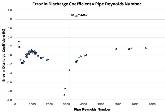
**Figure 13: Error in discharge coefficient versus Reynolds number for 8 inch  $\beta=0.6$  quadrant edge orifice plate**
