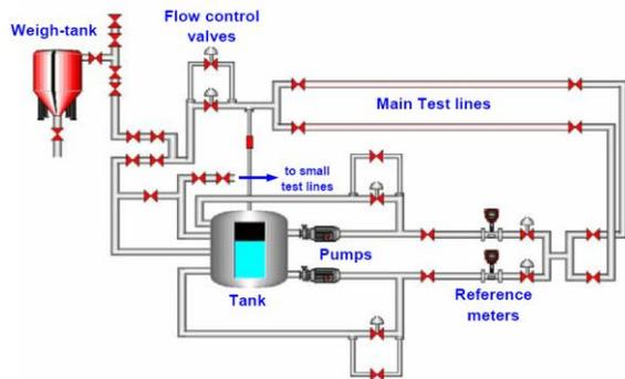
Figure 6: Schematic Diagram of the NEL Oil Flow Test Facility
