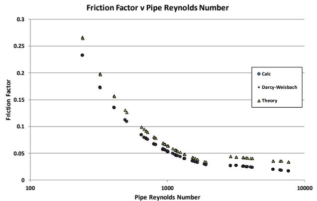
Figure 12: Friction factor versus Reynolds number for three different calculation methods
