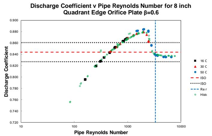
Figure 10: Discharge coefficient versus Reynolds number for 8 inch  $\beta=0.6$  QE orifice plate
