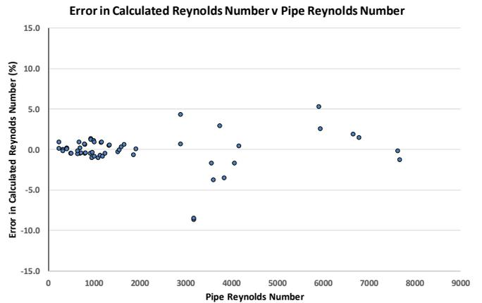
**Figure 14: Error in calculated Reynolds number versus Reynolds number for 8 inch  $\beta=0.6$  quadrant edge orifice plate**
