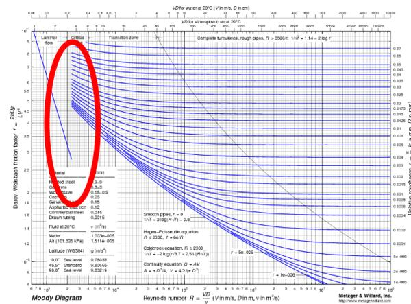
Figure 3: Darcy-Weisbach friction factor versus Reynolds number
