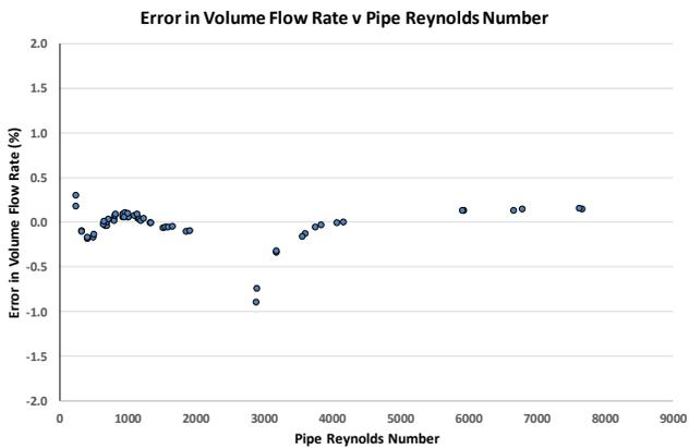
**Figure 15: Error in volume flow rate versus Reynolds number for 8 inch  $\beta=0.6$  quadrant edge orifice plate**
