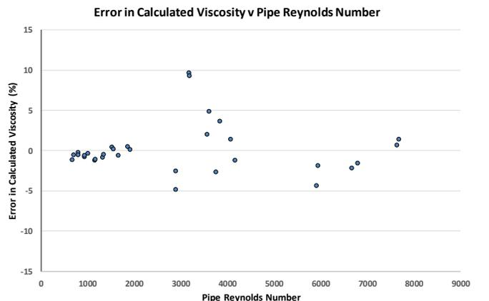
**Figure 18: Error in calculated viscosity versus Reynolds number for 8 inch  $\beta=0.6$  quadrant edge orifice plate**
