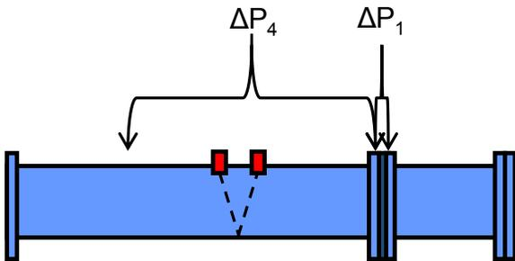
Figure 5: Orifice plate with additional clamp-on ultrasonic measurement (in red) upstream of primary element (flow left to right)
