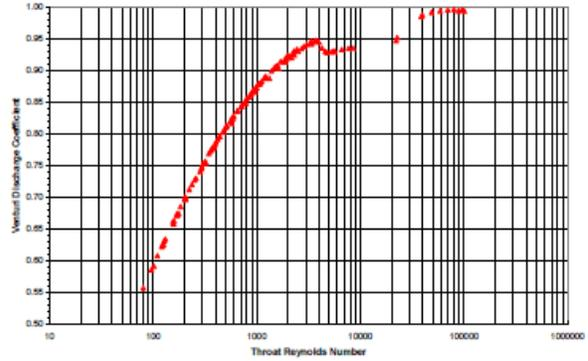
Figure 2: Typical discharge coefficient versus Reynolds number relationship
