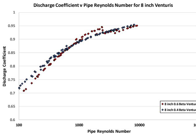
Figure 9: Discharge coefficient versus Reynolds number for 8 inch Venturis
