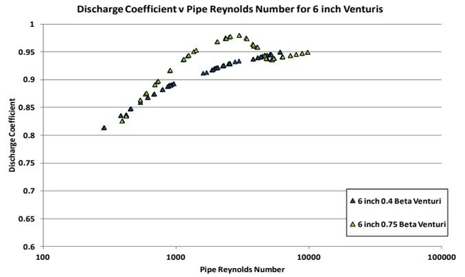
Figure 8: Discharge coefficient versus Reynolds number for 6 inch Venturis
