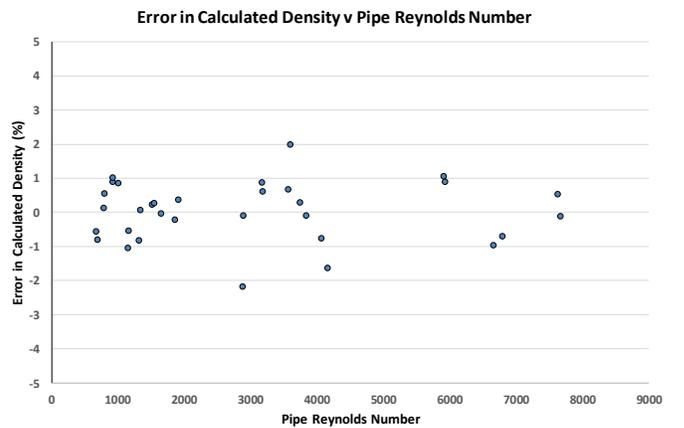
**Figure 16: Error in calculated density versus Reynolds number for 8 inch  $\beta=0.6$  quadrant edge orifice plate**
