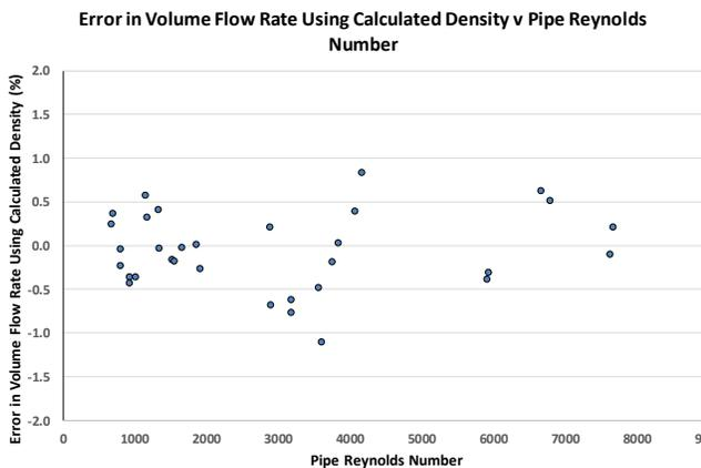
**Figure 17: Error in volume flow rate using calculated density versus Reynolds number for 8 inch  $\beta=0.6$  quadrant edge orifice plate**
