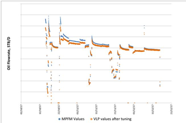
**Figure 11: Comparison between MPFM real time measurement and tuned VLP expression for well with higher curvature**
