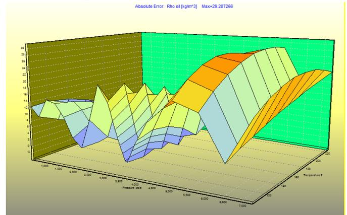
Figure 7: The difference between 3D surface of oil density predicted by EOS and 3D surface of oil density based on polynomial coefficients
