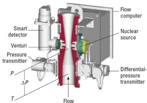
Figure 1: Simplified sketch of Vx (Source: Fundamentals of Multiphase Metering, Schlumberger).
