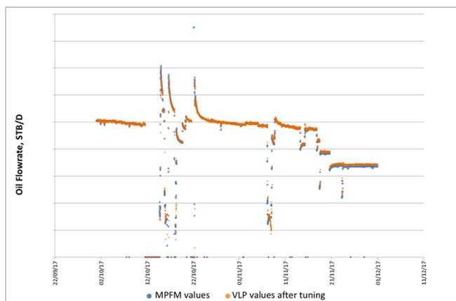
Figure 10: Comparison between MPFM real time measurement and tuned VLP expression for well with little curvature
