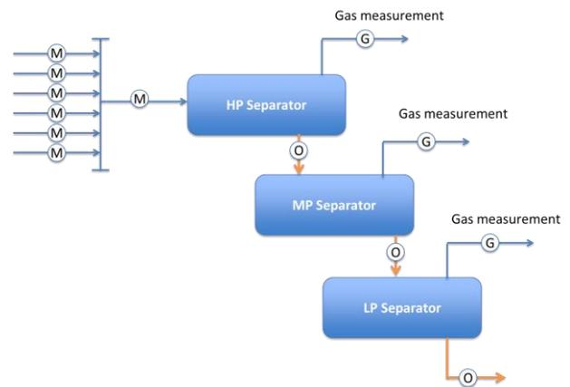
**Figure 9: Simplified schematic of separators and gas measurement**
