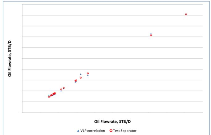
**Figure 13: Tuned VLP expression against Test Separator for well number 2**
