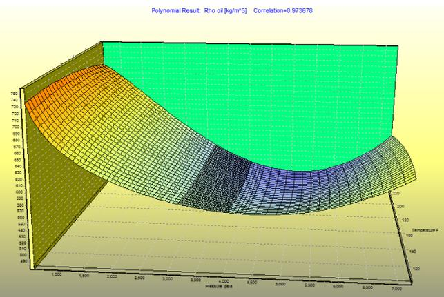
Figure 6: 3D surface of oil density based on sets of polynomial coefficients.
