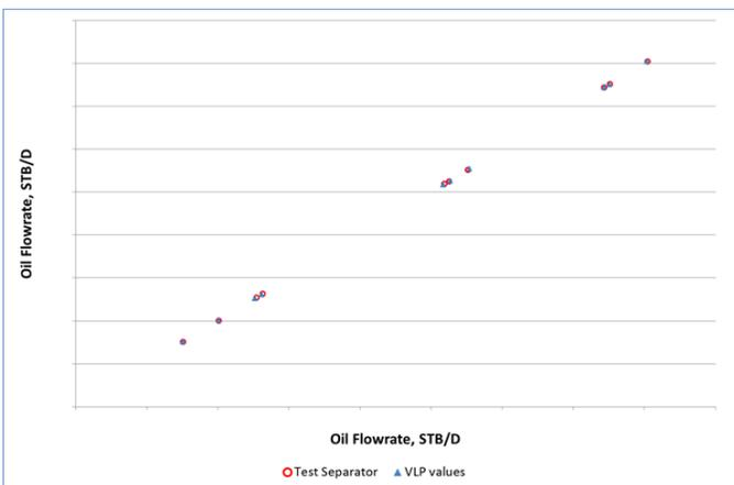
**Figure 12: Tuned VLP expression against Test Separator for well number 1**
