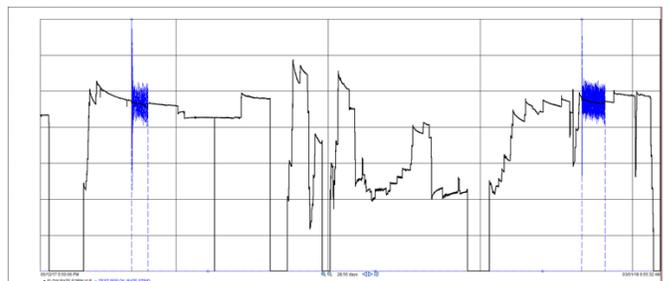
**Figure 15: VLP correlation values between two consecutive tests for well number 1. Blue line for test separator values, black line for VLP correlation trend. Y axis = oil flow rate.**
