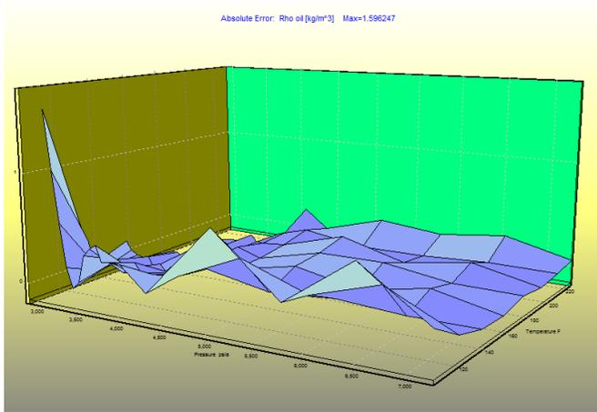
**Figure 8: The difference between 3D surface of oil density predicted by EOS and 3D surface of oil density based on polynomial coefficients after splitting the polynomial into above and below bubble point**
