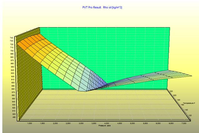
Figure 5: 3D surface of oil density based on EOS
