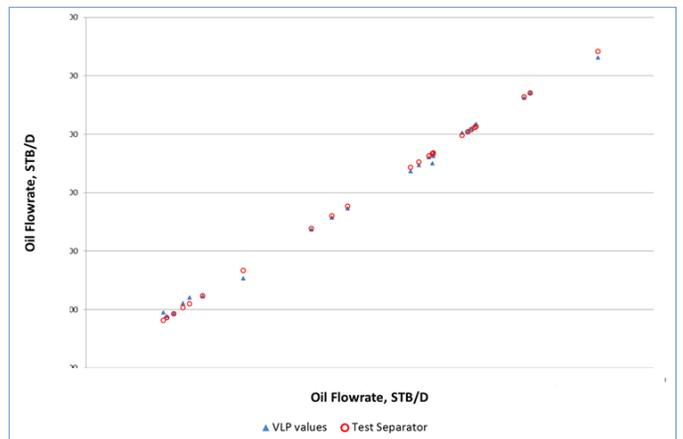
**Figure 14: Tuned VLP expression against Test Separator for well number 3**
