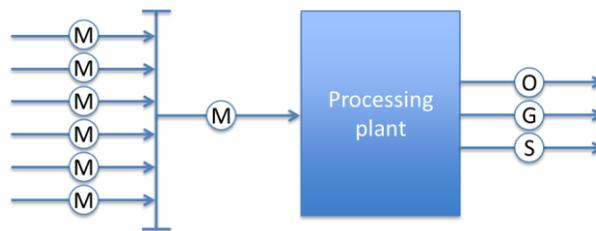
Figure 3: Simplified Allocation scheme. M: multiphase flow, G: gas, O: liquid, S: sulphure
